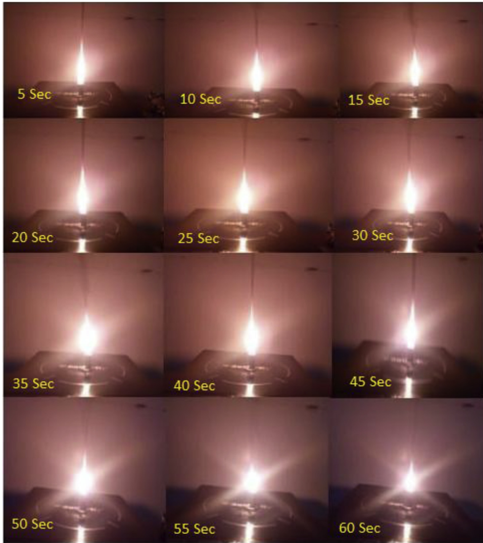
Fig. 7. Benzoic resin exhibiting a laminar short length flame at 270°C surface temperature.
